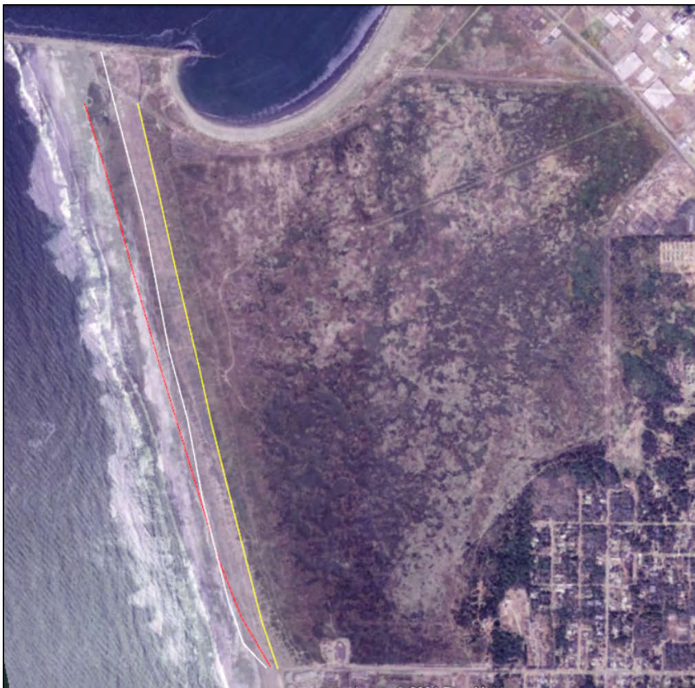
Figure 7. Shoreline retreat from 1974-2016 along the western boundary of Westport Light State Park. Red=1974, White=1985, Yellow=2016. Underlying imagery is from 1974 (USGS Earth Explorer).
