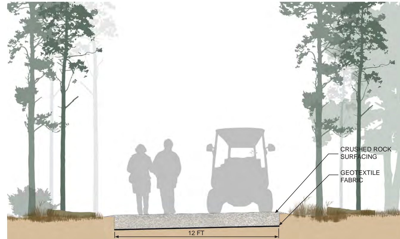
CRUSHED ROCK SHUTTLE SERVICE PATH
