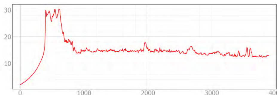
Figure 5. Topographic profile of a representative west-east transect across Westport Light State Park. Axes are in feet. Beginning at the ocean, the beach gradually increases in elevation to approximately 16 feet, where the 10-foot high vertical bluff of the stabilized foredune is encountered. Slightly rolling topography atop the foredune includes the cement walking path, east of which the deflation plain begins. Profile created from 2019 Lidar data obtained from WA DNR on 1/28/21.
